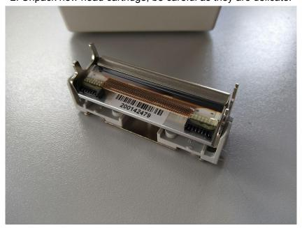
Note that the head cartridge has a grey plastic cage, **each side** is held in place with a flexible tang that clips into the lid of the printer, these are all that hold it in place, there are no screws.
