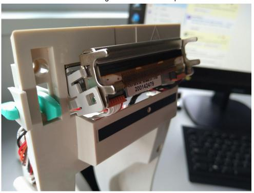
6: With the head back inplace you are ready to test it, turn it on as normal and test a label print.
