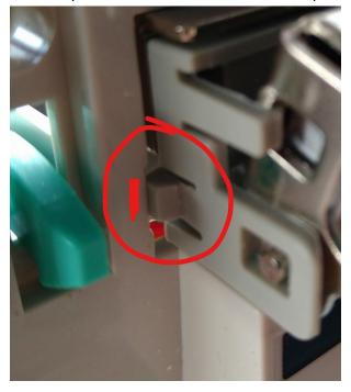
3: Carefully insert the screwdriver into this gap as shown, and prize sideways, this should bend the tang inwards and the head should start to move out of its slot, do the same to both sides and carefully work the head loose. BE CAREFUL not to damage the 2 electrical connectors.
