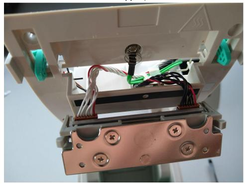
5: Connect the new head to the electrical connectors and re-align and push the head back into its slot, you may need to slightly bend in the grey plastic tangs on the new head with the screwdriver to get it to click back in place.
