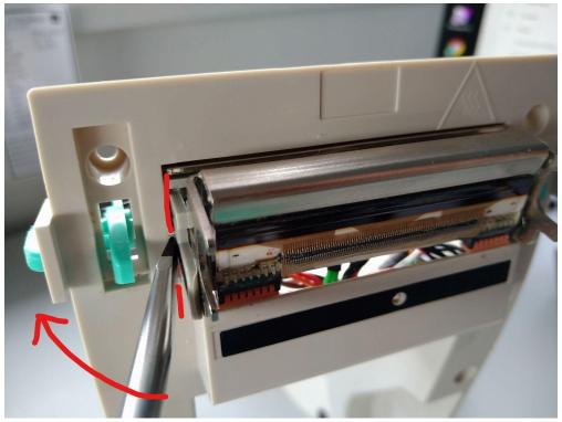
4: The head should now be loose as such, now you can carefully disconnect both electrical connectors, they just pull out.
