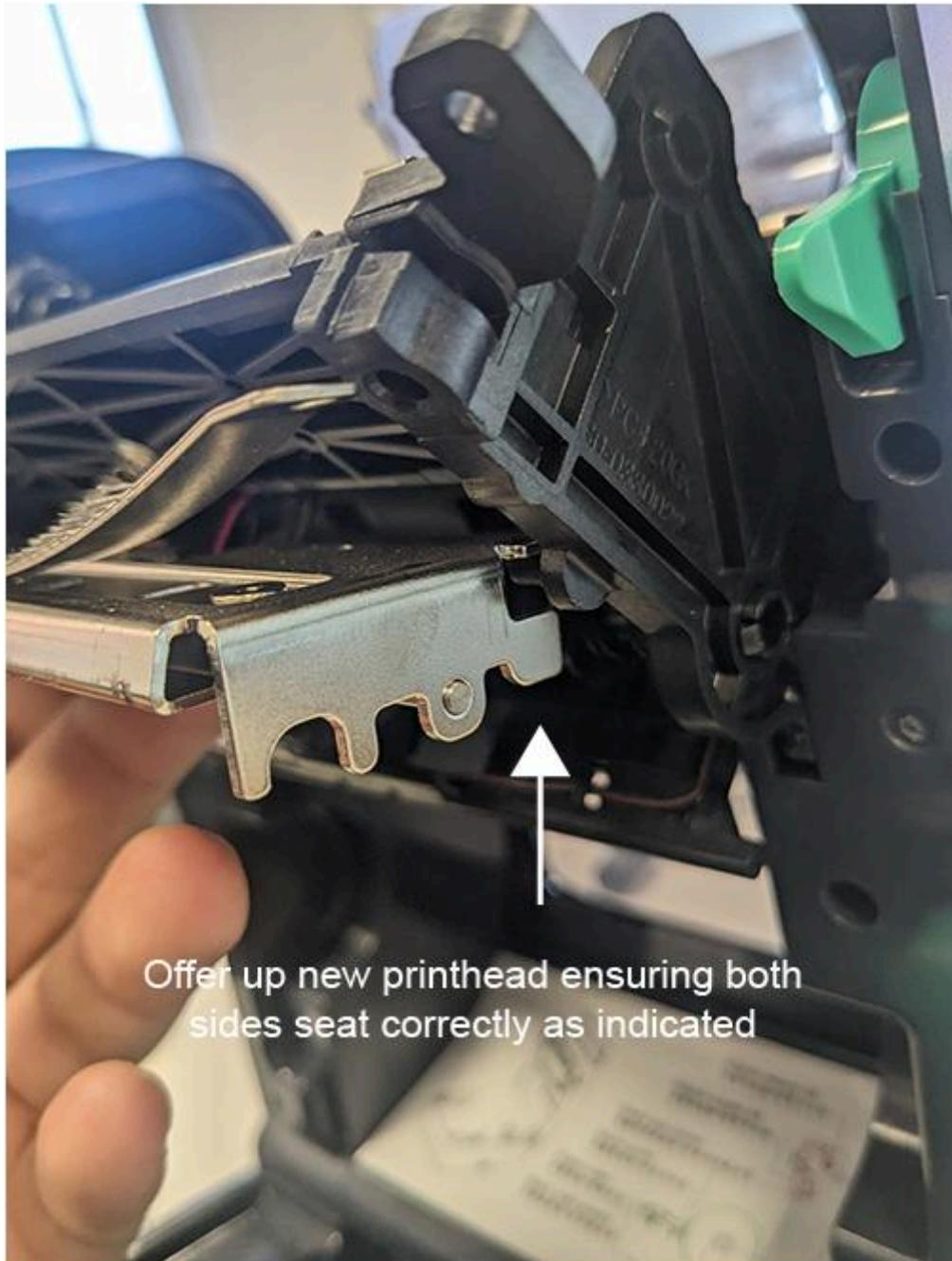
Step 13: Offer up the leaf spring component into retaining gap and push back to seat correctly.
