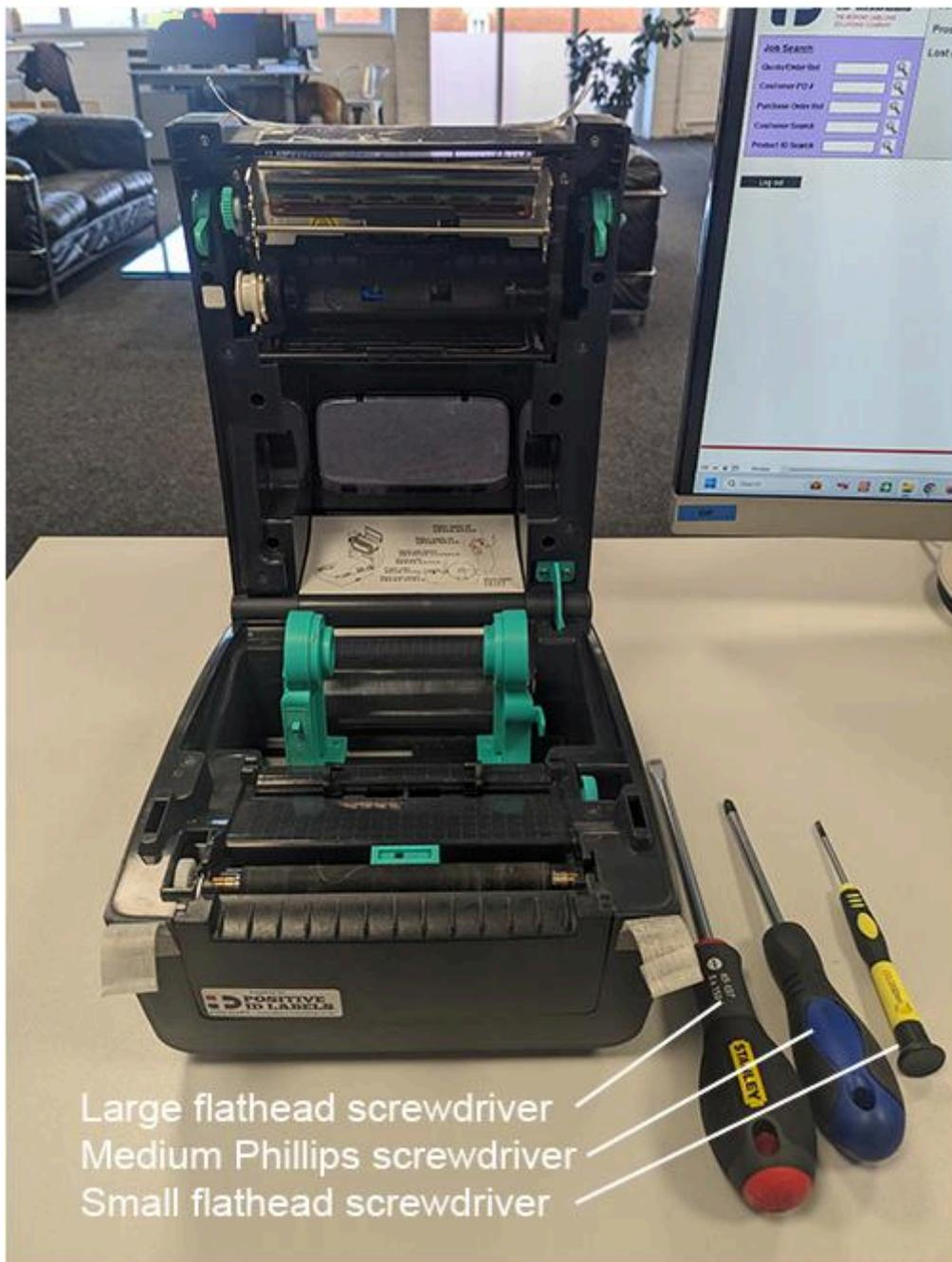
Step 2: Position the printer resting on the rear of the clamshell to ease access.
