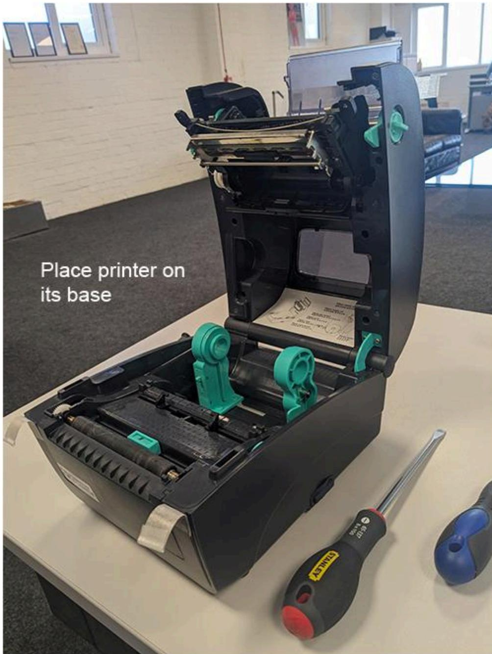
Step 8: Open thermal printer ribbon cover to allow the printhead assembly to drop
